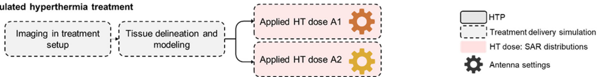
Figure 5. Description of the three plans (plan A1, A2 and B) and the applied HT dose during the simulated hyperthermia treatment (applied HT doses A1 and A2). Plan A1 starts with obtaining the patient data without the MR-compatible hyperthermia device. After tissue delineation and generation of the 3D patient model are performed, SAR-based optimization in which antenna settings are defined. In the last step of the HTP, the SAR distributions are obtained (dose predictions) using the optimized antenna settings. Plan A2 follows the same steps; however, rigid registration is performed to adjust the MR images from the planning position to the treatment position (Figure 4b). In Plan B, the volunteer is scanned with the MR-compatible hyperthermia device and a filled water bolus (treatment setup). In the simulated hyperthermia treatment, the applied HT dose was calculated using Plan A1 and Plan A2 antenna settings. Five SAR distributions were obtained, where three represent the dose predictions from the treatment plans, and two denote the applied HT dose in the simulated treatment. The symbol's color of the antenna settings denotes the plan in which these were optimized. Overall, Plan A1 and A2 represent the current HTP, Plan B is the idealized treatment plan, and Applied HT doses A1 and A2 denote the current treatment in clinical practice.
