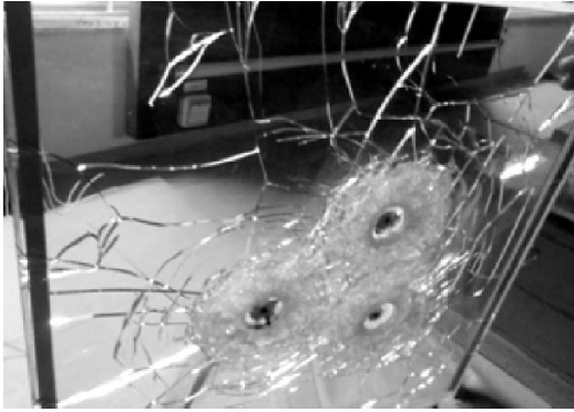
Fig. 3. Fracture of the slab of protective HS-glass.
