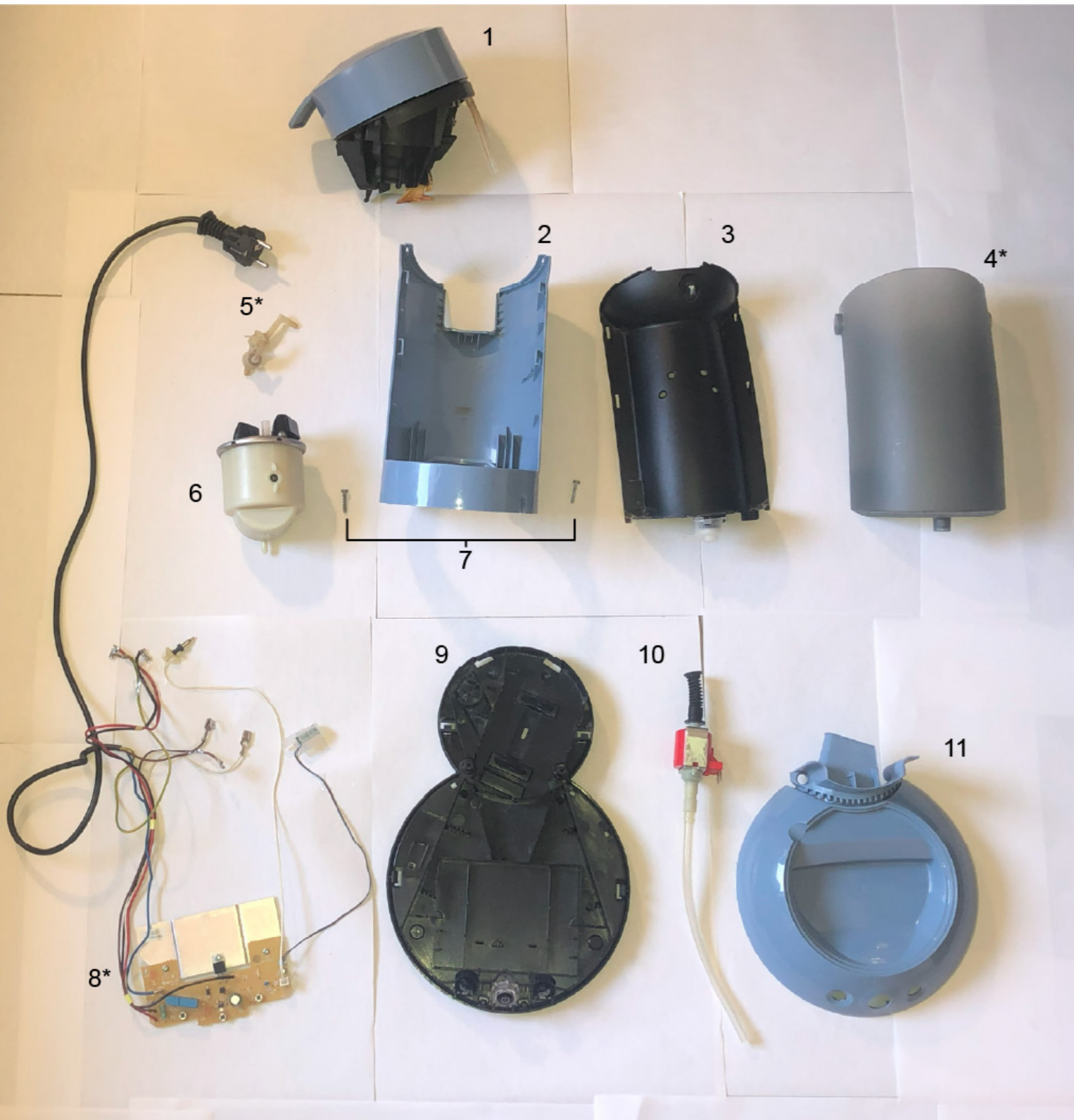
Figure 37: Exploded side view of a Senseo HD7817 existing out of recognisable subassemblies (numbers correspond to Table 6; '*' are the critical parts)
