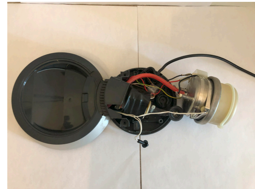
Figure 39: Wires and tubes are covered by drip tray shell
