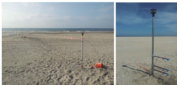
Figure 3: Measurement setup of masts with the wind speed and direction sensor and laser sensors
