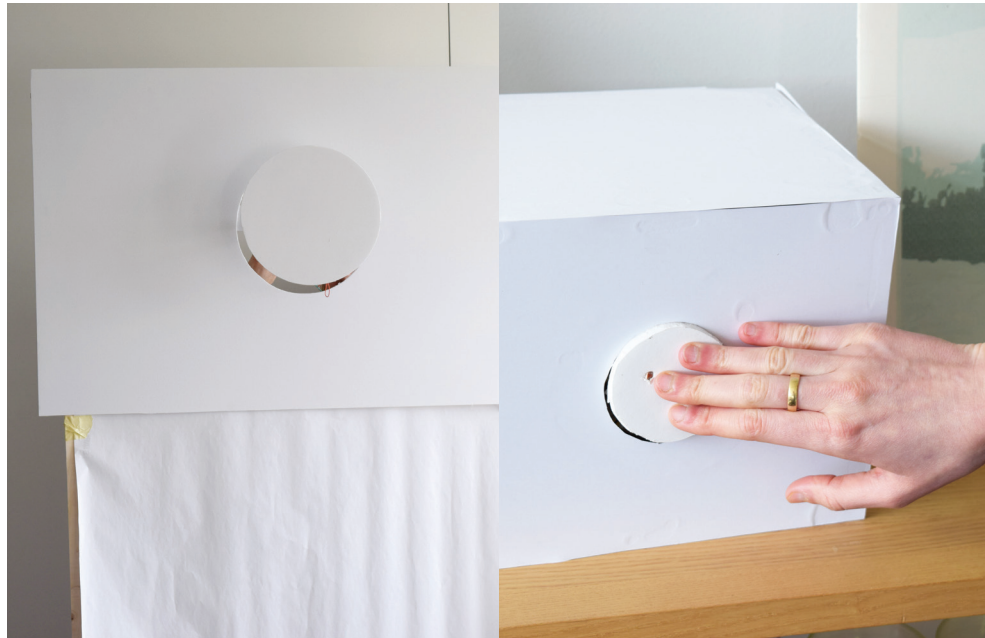
Fig. 51 - The prototype of the feedback valve includes a control and a valve. The two are a form family and indicate the systems' activity by the position. The interaction of the control works using an arduino and a solenoid.
