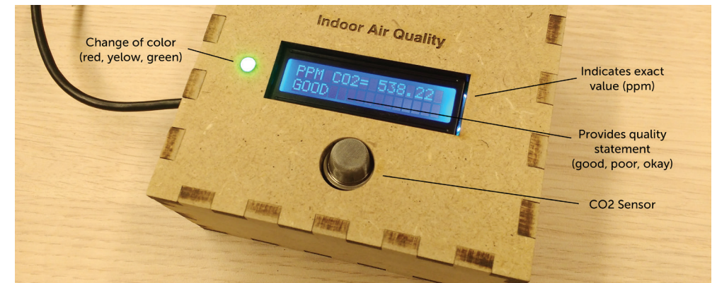
Fig. 38 - The probe communicates air quality in various ways. The aim of the probe is to learn how people experience real-time feedback on air quality
