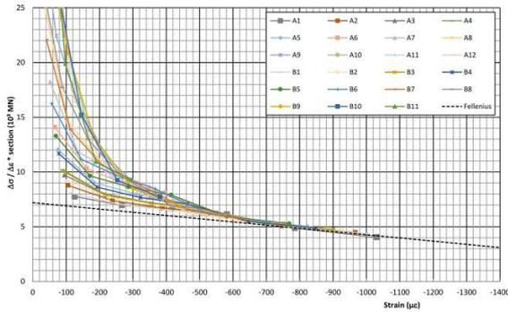
Figure 6. EA according to Fellenius for SLT 2
