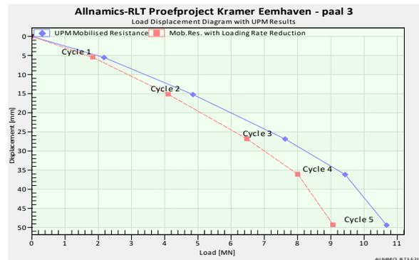
Figure 11. Load-settlement graph RLT at pile P3
