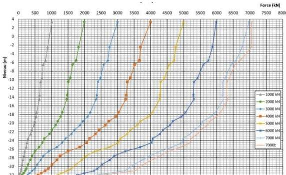
Figure 7. Force distribution along the pile for SLT 2
