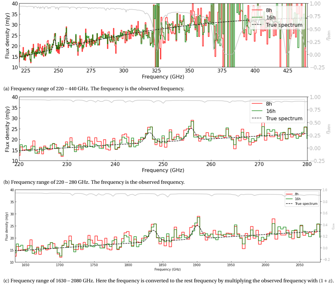
Figure 4.9: TIEMPO simulation of HFLS3 with the flux density in mJy vs the frequency in GHz. In the plot the red line is a simulation of 8 hours and the green line a simulation of 16 hours. For both simulations the pwv value is 1.0 mm. The black dashed line is the expected spectrum of HFLS3, smoothed to account for the resolving power of the spectrometer. The flux density is obtained by subtracting the centre off data from the centre on data, and corrected for the atmosphere transmission.
