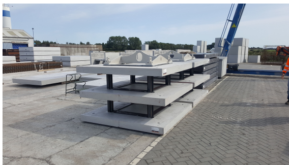
Figure 5.12: Manufactured oyster broodstock structure with flat, solid plates
