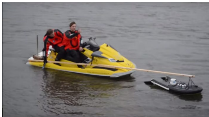
Figure 8 set-up: Jet-ski with the attached ADCP
