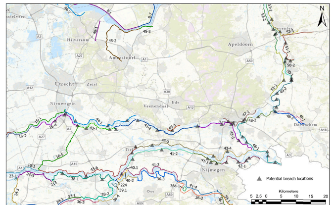
Fig. 7. Segments (coloured and numbered lines) and breach locations (grey triangles) in the study area.
