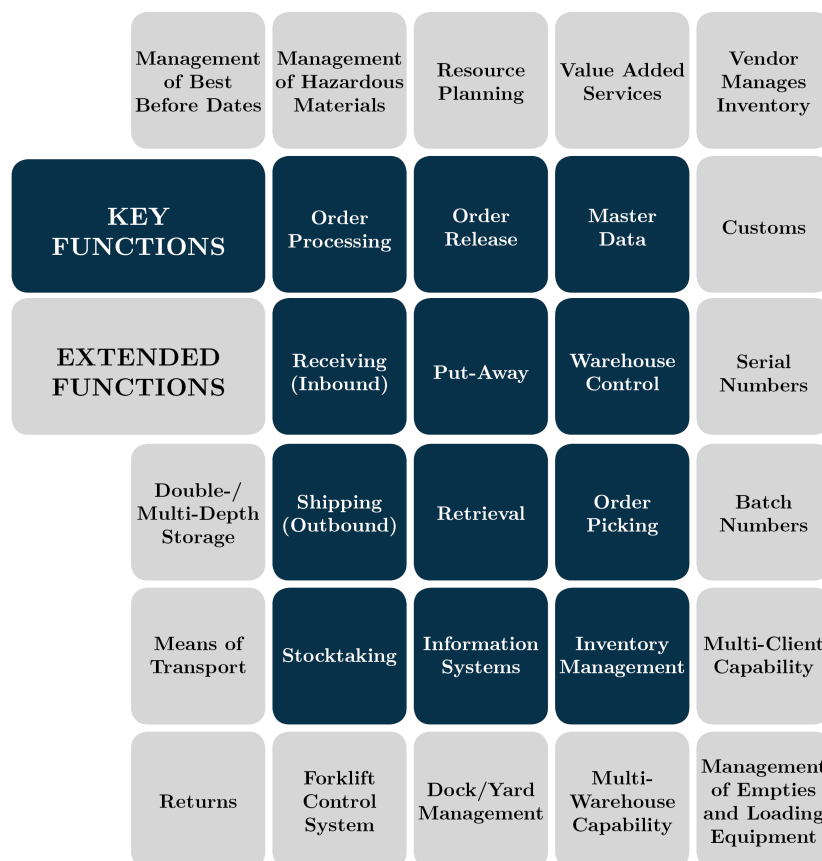
Figure B-3: Key and extended functionality of typical WMS systems (adapted from Nettsträter et al., 2015, p.5)
