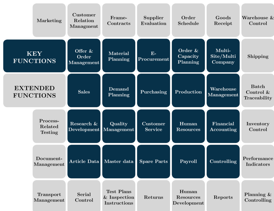
Figure B-1: Key and extended functionality of typical ERP systems (adapted from Nettsträter et al., 2015, p.3)
