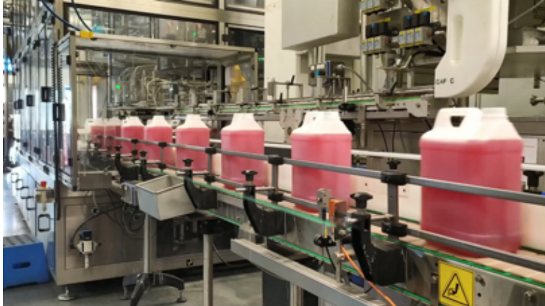
Figure 1.3: Filled detergent canisters exiting the filling and capping machine in an agile factory.
