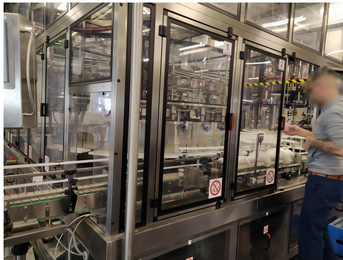
Figure 1.1: A factory operator solving a problem with one of the machines along a detergent production line
