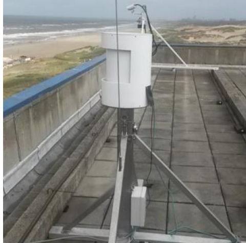
Figure 3.2: Riegl VZ2000 laser scanner mounted on the roof of a hotel facing the coast of Kijkduin, the Netherlands. The scanner is covered with a protective case to shield it from wind and rain.
