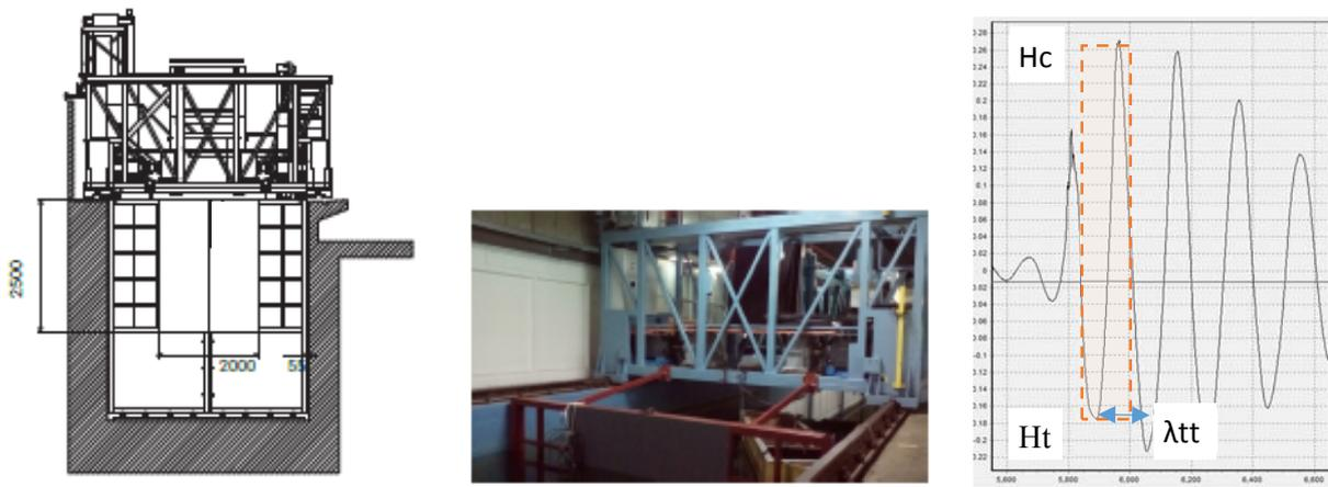
Figure 3: a) View of test set-up from the wave generator: A wall, mounted on a steel frame, extends 0.6 m above water; b) A wave group as used with the running-up wave marked.
