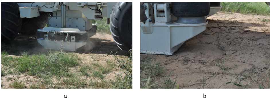
Figure 3.12: Photos taken at the second location. Showing (a) dust clouds at the high end of the sweep and (b) small heaps next to plate and air gaps between the plate and ground.
