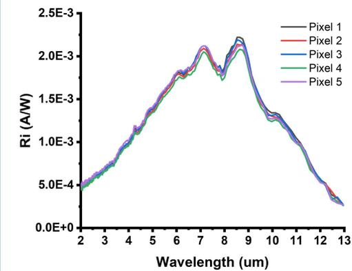
Fig. 5. Low frequency spectral characteristics of individual pixels.
