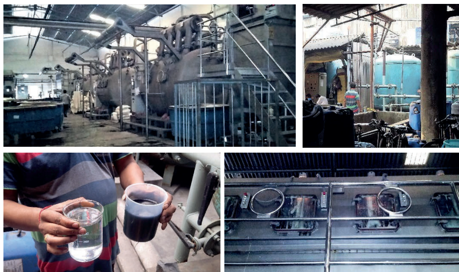
Figure 8.4 Dyeing factory in Badai village. Clockwise from top left: Scale of factory operations; On-site effluent treatment plant; Automated dyeing machines; Difference in effluents before and after treatment (Photos courtesy Gomes, 2016).
