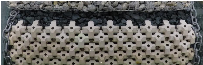
Figure H-13: Test series 1.1.2 Initial – Before Test with N_s=1.45 (60% design conditions)
