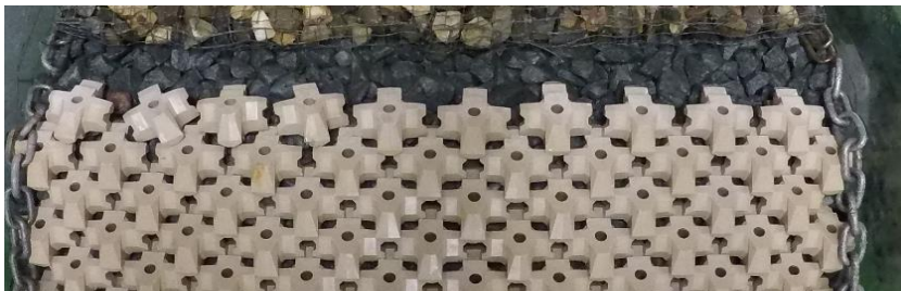
Figure H-98: Test series 1.1.3 Repetition – Before Test with N_s=2.55 (100% design conditions)
