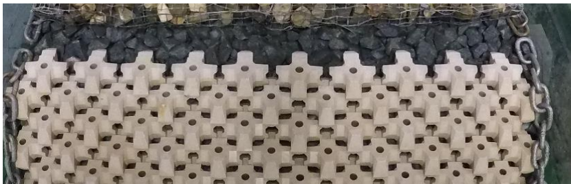
Figure H-93: Test series 1.1.3 Repetition – Before Test with N_s=1.22 (50% design conditions)
