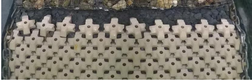
Figure H-70: Test series 1.1.2.1 Repetition – Before Additional Test with N_s=3.10 (120% design conditions)
