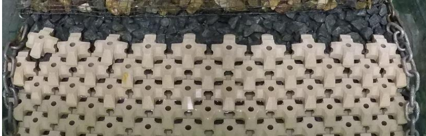
Figure H-86: Test series 1.2.2 Repetition – Before Test with N_s=1.69 (70% design conditions)
