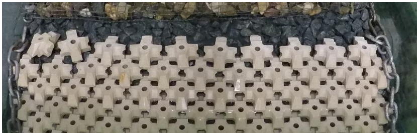
Figure H-89: Test series 1.2.2 Repetition – Before Test with N_s=2.42 (100% design conditions)
