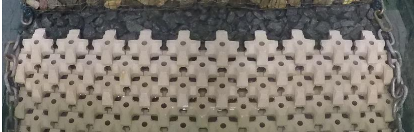
Figure H-71: Test series 1.1.2 Repetition – Before Test with N_s=0.73 (30% design conditions)
