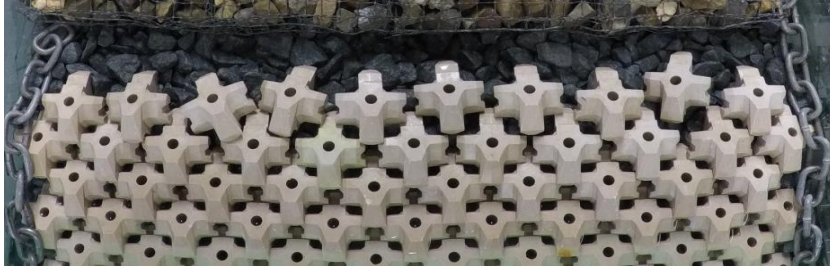
Figure H-16: Test series 1.1.2 Initial – Before Test with N_s=3.09 (120% design conditions)
