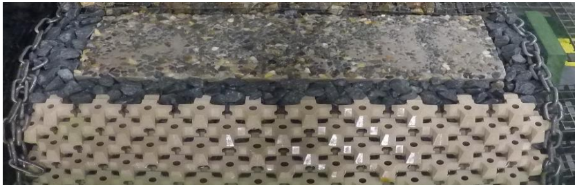
Figure H-148: Test series 6.2.2 – After Test with N_s=3.55 (140% design conditions)
