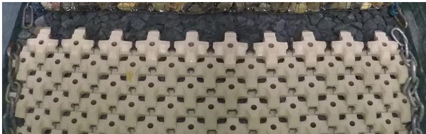
Figure H-48: Test series 1.1.1 Repetition – Before Test with N_s=0.98 (40% design conditions)
