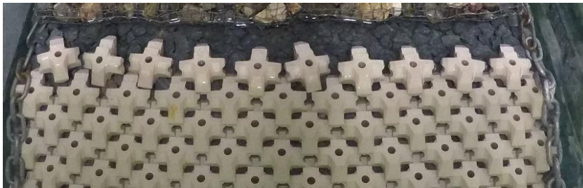
Figure H-69: Test series 1.2.1 Repetition – Before Additional Test with N_s=3.10 (120% design conditions)
