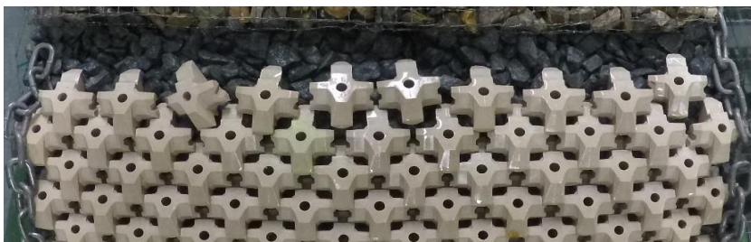
Figure H-29: Test series 1.1.3 Initial – After Test with N_s=3.10 (120% design conditions)
