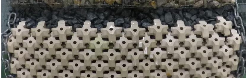
Figure H-35: Test series 1.2.3 Initial – After Test with N_s=3.07 (120% design conditions)
