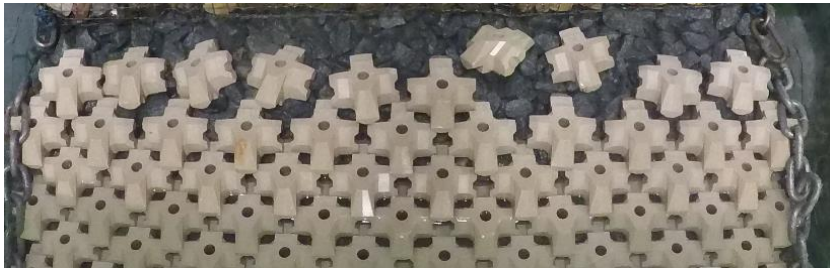
Figure H-78: Test series 1.1.2 Repetition – Before Test with N_s=2.44 (100% design conditions)
