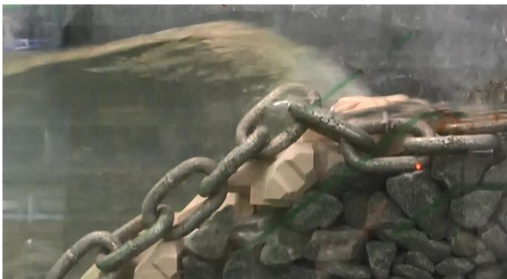
Figure 5.6: Collapsing breaker at the top armour row
