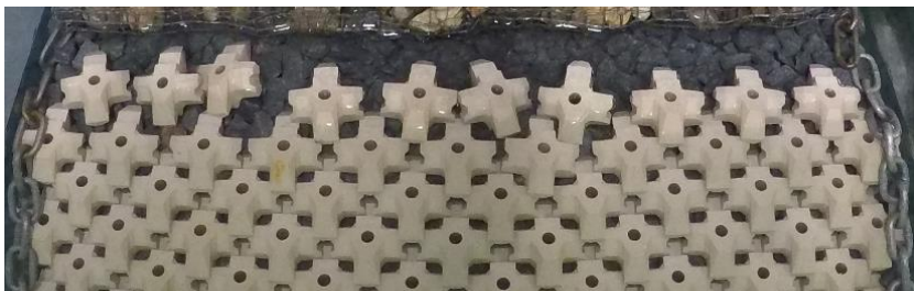
Figure H-59: Test series 1.2.1 Repetition – Before Test with N_s=0.74 (30% design conditions)
