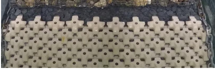
Figure H-65: Test series 1.2.1 Repetition – Before Test with N_s=2.25 (90% design conditions)
