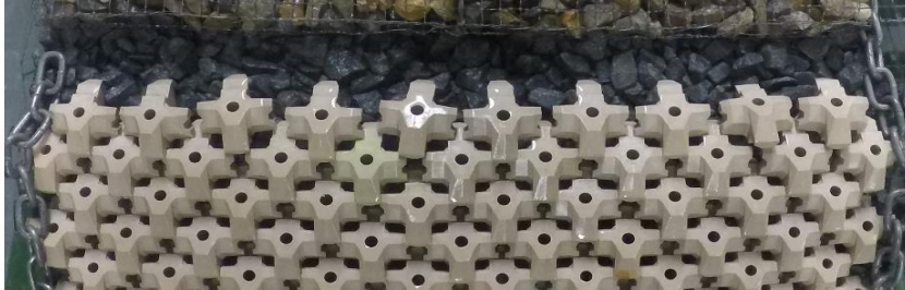
Figure H-46: Test series 1.2.4 Initial – After Test with N_s=3.33 (120% design conditions)
