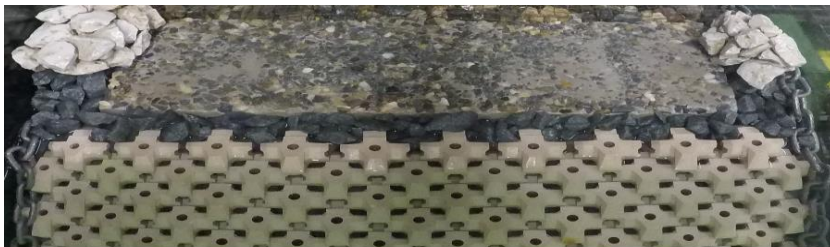
Figure H-132: Test series 6.2.1 – Before Test with N_s=1.96 (80% design conditions)
