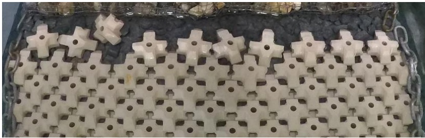
Figure H-62: Test series 1.2.1 Repetition – Before Test with N_s=1.50 (60% design conditions)
