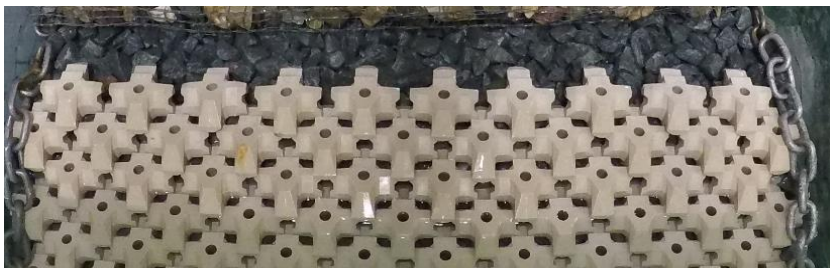
Figure H-84: Test series 1.2.2 Repetition – Before Test with N_s=1.28 (50% design conditions)
