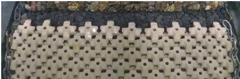
Figure H-54: Test series 1.1.1 Repetition – Before Test with N_s=2.47 (100% design conditions)
