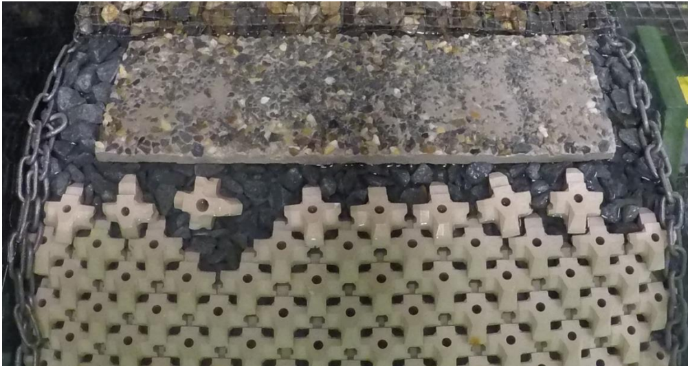
Figure 4.11: Armour layer at the end of test series 6.1.1
