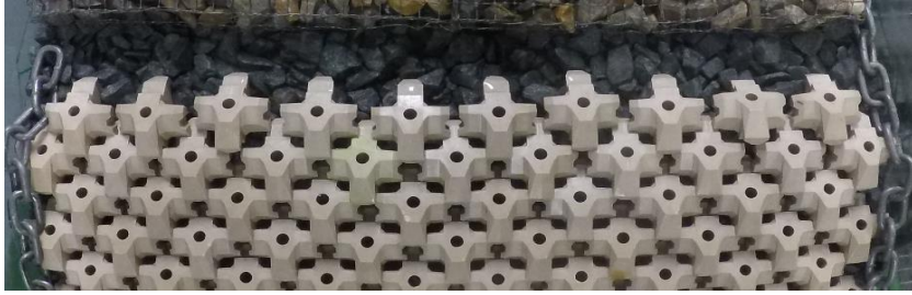
Figure H-40: Test series 1.1.4 Initial – After Test with N_s=2.97 (120% design conditions)
