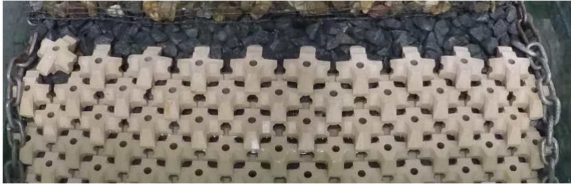
Figure H-87: Test series 1.2.2 Repetition – Before Test with N_s=1.96 (80% design conditions)
