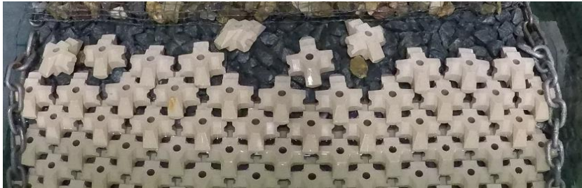
Figure H-91: Test series 1.2.2 Repetition – Before Test with N_s=2.97 (120% design conditions)
