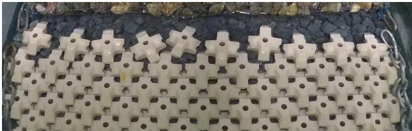
Figure H-49: Test series 1.1.1 Repetition – Before Test with N_s=1.23 (50% design conditions)
