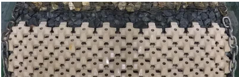
Figure H-94: Test series 1.1.3 Repetition – Before Test with N_s=1.49 (60% design conditions)
