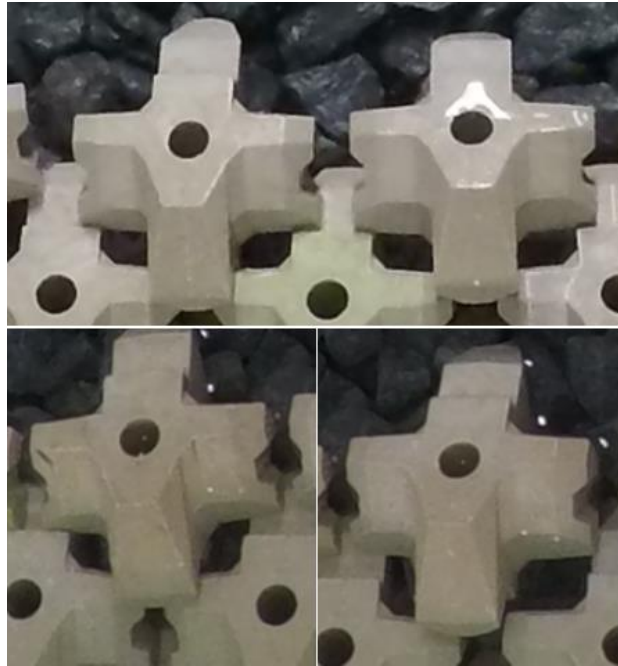
Figure 2.10: Top left: Stable unit; Top right: Stage 1 of partial displacement; Bottom left: Stage 2 of partial displacement; Bottom right: Stage 3 of partial displacement
