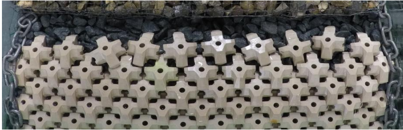
Figure H-17: Test series 1.1.2 Initial – After Test with N_s=3.09 (120% design conditions)
