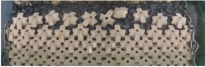
Figure H-80: Test series 1.1.2 Repetition – Before Test with N_s=3.17 (120% design conditions)
