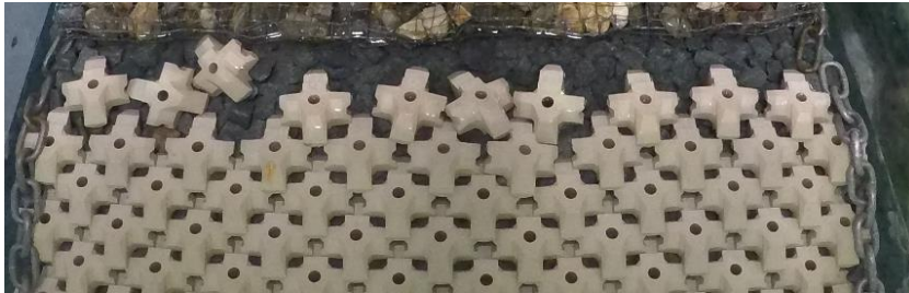
Figure H-61: Test series 1.2.1 Repetition – Before Test with N_s=1.26 (50% design conditions)
