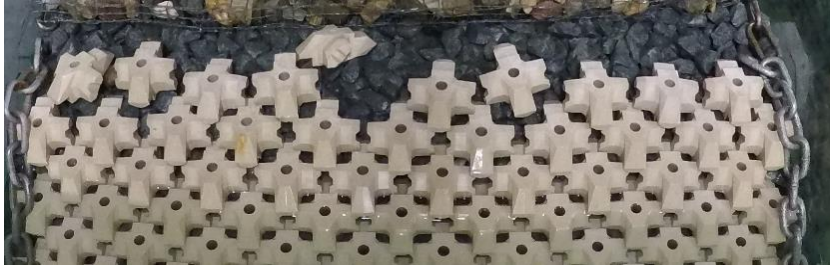
Figure H-90: Test series 1.2.2 Repetition – Before Test with N_s=2.66 (110% design conditions)
