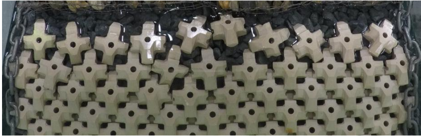
Figure H-12: Test series 1.2.1 Initial – After Test with N_s=3.11 (120% design conditions)
