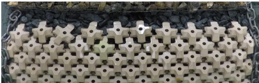
Figure H-23: Test series 1.2.2 Initial – After Test with N_s=3.07 (120% design conditions)
