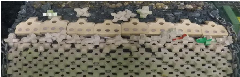
Figure H-118: Test series 5.2.1 – After Test with N_s=3.54 (140% design conditions)
