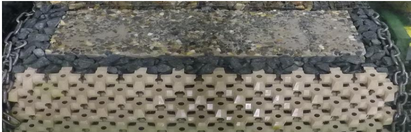
Figure H-141: Test series 6.2.1 – Before Test with N_s=3.38 (140% design conditions)
