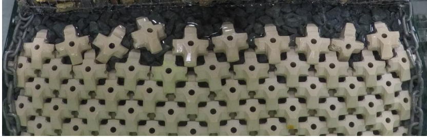
Figure H-6: Test series 1.1.1 Initial – After Test with N_s=3.17 (120% design conditions)
