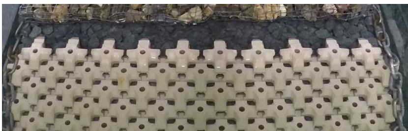
Figure H-64: Test series 1.2.1 Repetition – Before Test with N_s=1.90 (80% design conditions)
