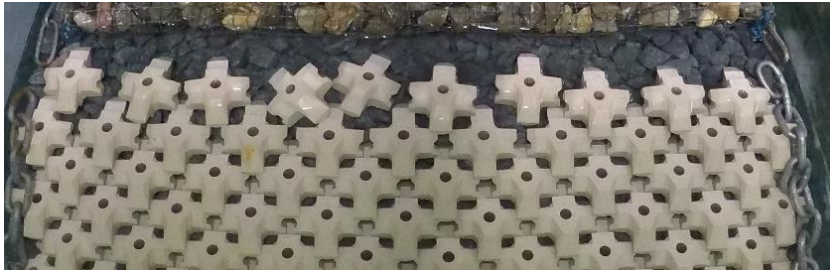
Figure H-50: Test series 1.1.1 Repetition – Before Test with N_s=1.48 (60% design conditions)
