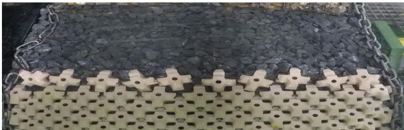
Figure H-123: Test series 7.2.1 – After Test with N_s=2.75 (110% design conditions)
