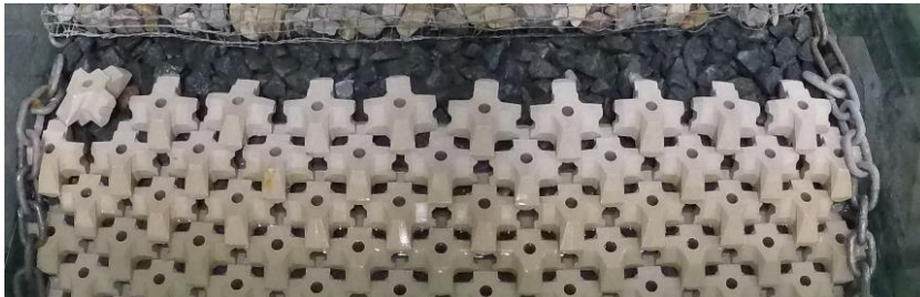
Figure H-88: Test series 1.2.2 Repetition – Before Test with N_s=2.29 (90% design conditions)
