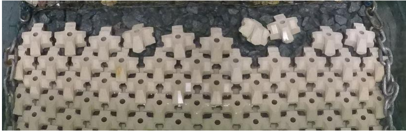
Figure H-77: Test series 1.1.2 Repetition – Before Test with N_s=2.28 (90% design conditions)
