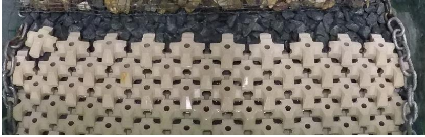
Figure H-85: Test series 1.2.2 Repetition – Before Test with N_s=1.48 (60% design conditions)
