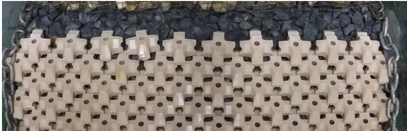
Figure H-96: Test series 1.1.3 Repetition – Before Test with N_s=2.06 (80% design conditions)
