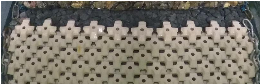
Figure H-53: Test series 1.1.1 Repetition – Before Test with N_s=2.21 (90% design conditions)
