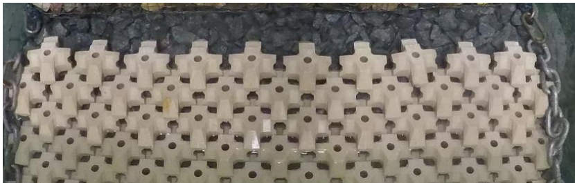
Figure H-74: Test series 1.1.2 Repetition – Before Test with N_s=1.50 (60% design conditions)
