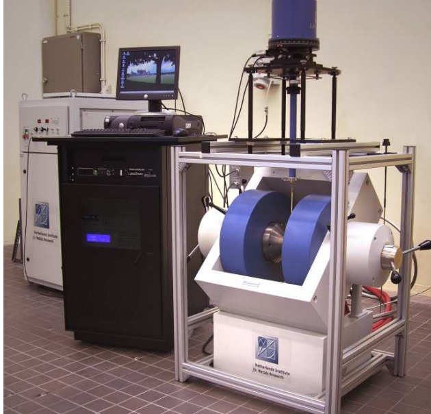
Figure 3.3 Lake Shore 7307 Vibrating Sample Magnetometer with room temperature set-up.
