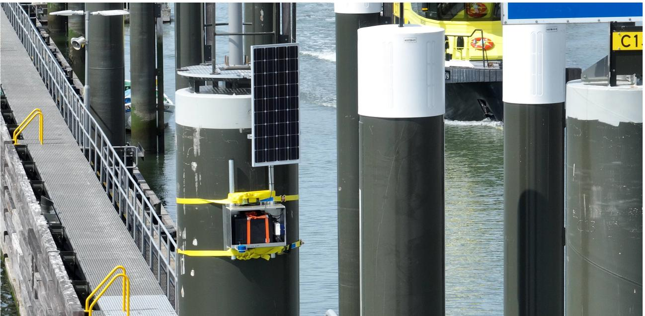
Figure A.5: Radar measurement device installed in the outer harbour of the Hansweert lock.
