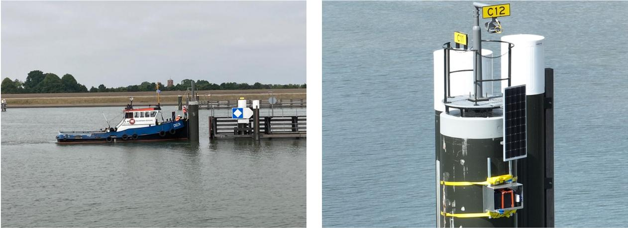
Figure C.2: Pictures of the installation and configuration of the water level fluctuation measurement setup.
