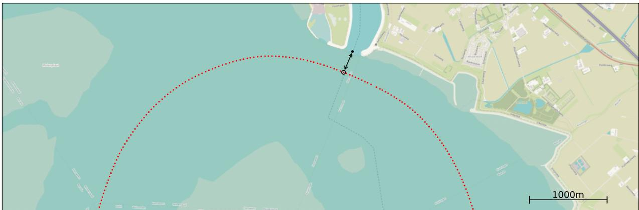
Figure 4.7: Plot showing the track of the coordinates of the middle of an arbitrary vessel passage. The definition of time of passage and passing distance is based on the coordinate with the smallest distance to the harbour entrance.
