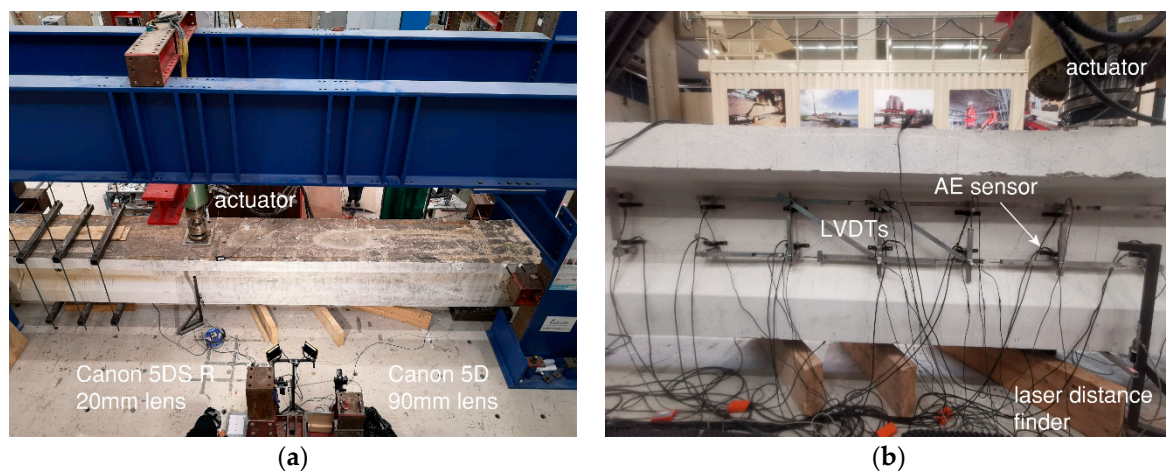
Figure 1. Overview of test setup: (a) At DIC side, and (b) at sensor side.
