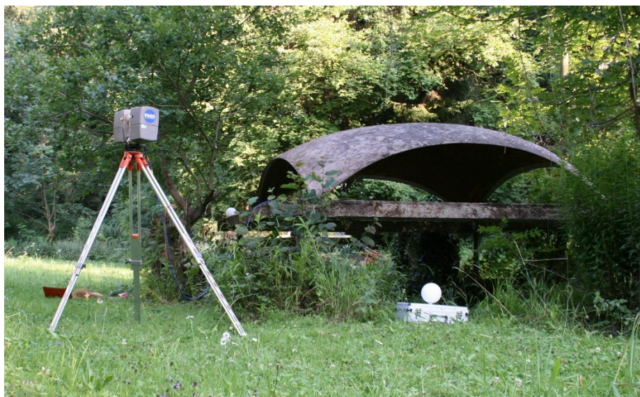
Figure 8 scanning of the Bellinzona shell model of Heinz Iser, Burgdorf, Switzerland by team from TU Delft, July 2011
