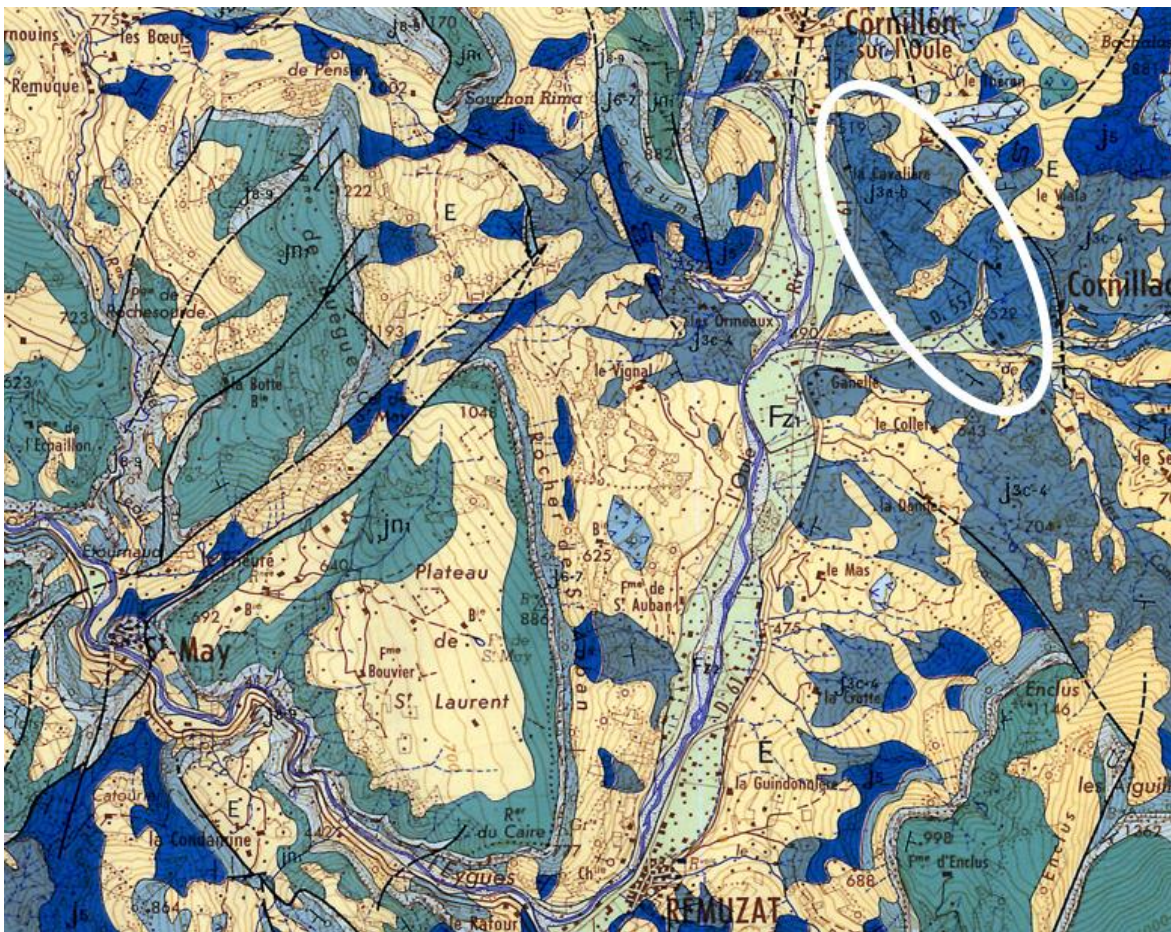
Fig.59: Geological map of the BRGM showing the older formation (encircled in white) of the Terres Noires compared to the surrounding Terres Noires formation.
