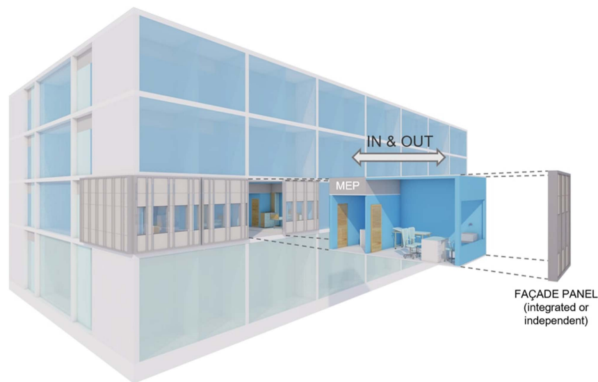
Fig. 7. MAHD system diagram—with the details of the superstructure and the inserted modules.
