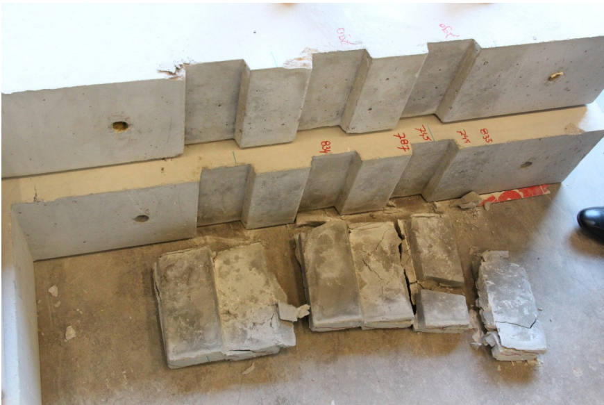
Figure E.5: Specimen 2-7: Dismantled specimen (Tiksomortar K70)
