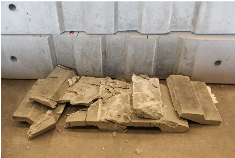
Figure E.3: Specimen 1-3: Dismantled specimen (Tiksomortar k70)
