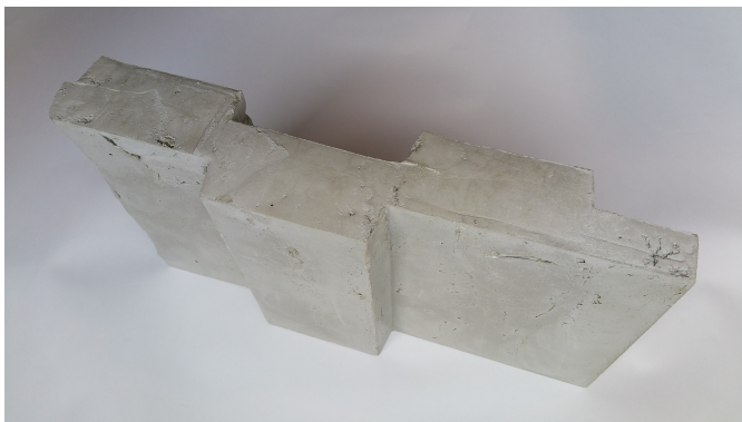
Figure 4.3: The mortar filling after demoulding
