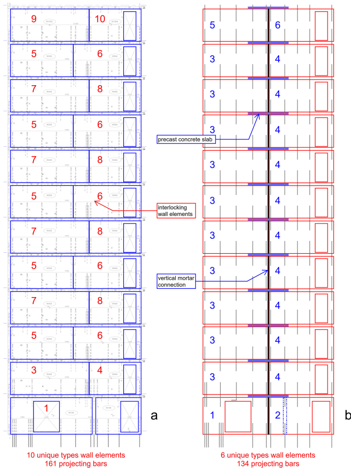
Figure 8.3: Precast concrete cantilever shear wall designs with traditional interlocking element lay-out (a) and a version with a vertical mortar connection (b)
