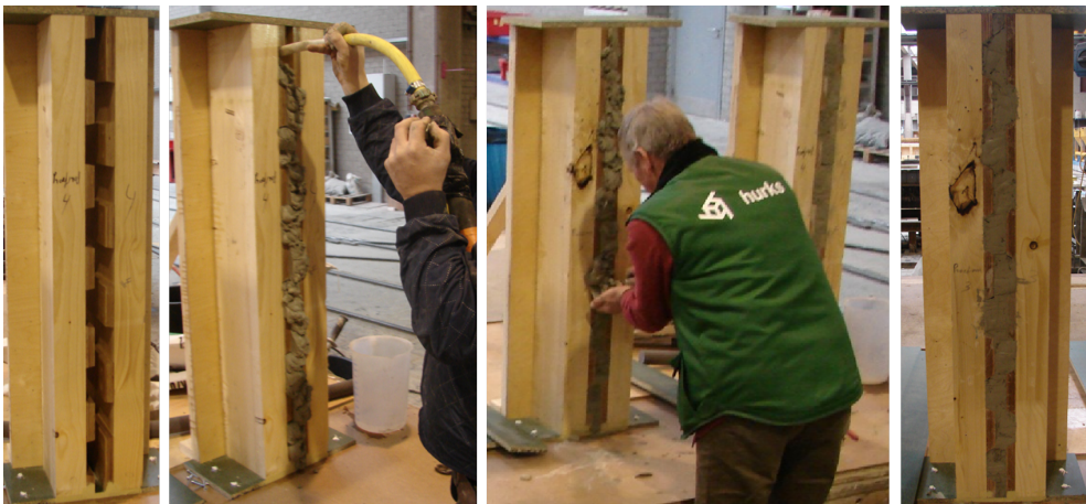
Figure 1.5: Testing the filling of vertical seams with a mortar pump
