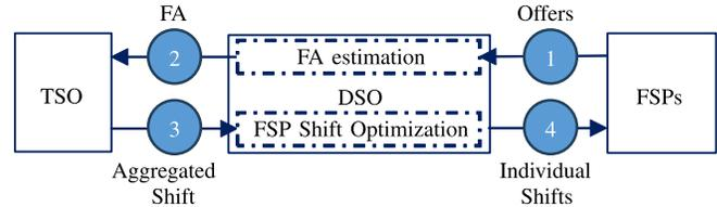
Fig. 1. DSO-managed approach for TSO-DSO Coordination. Steps order (1).
