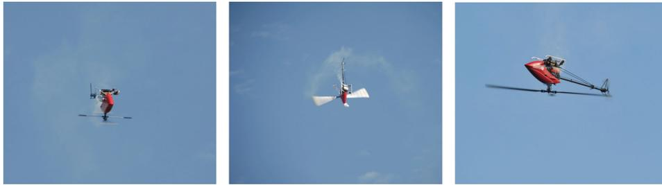
Figure 2.12: Snapshots of the autonomous helicopter acrobatics [41]
