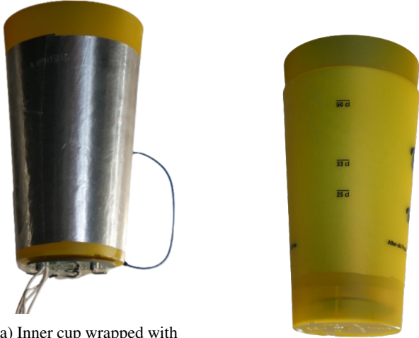
(a) Inner cup wrapped with aluminium foil for capacitive touch sensing
