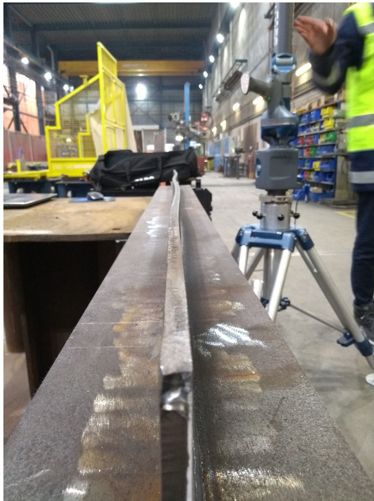
Figure A.9: Post welding deformation clearly visible with naked eye
