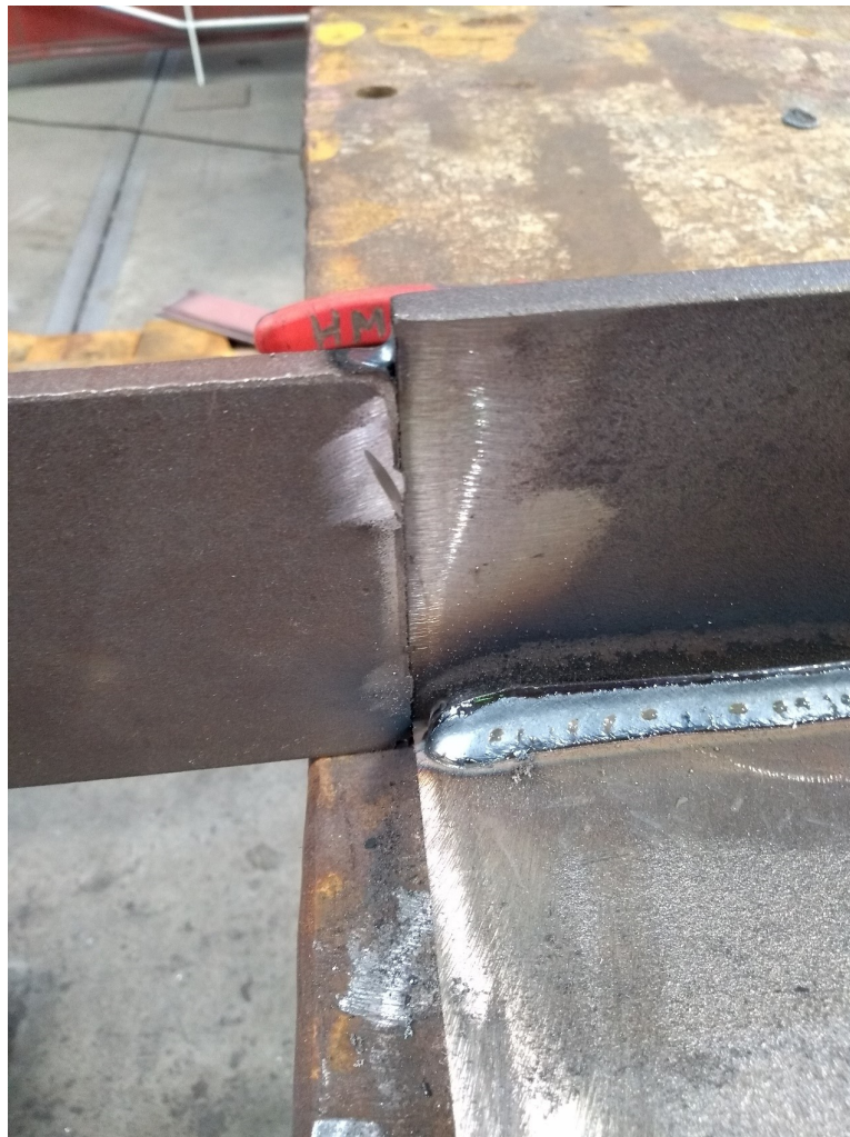
Figure A.6: Boundary condition of one edge of specimen during welding
