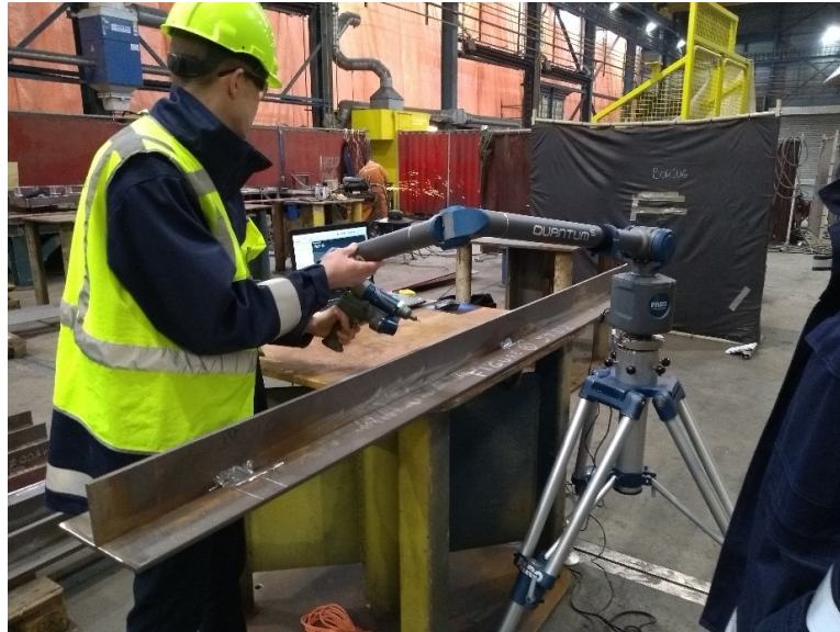
Figure 3.5: Faro measurement arm and operator in action during scanning
