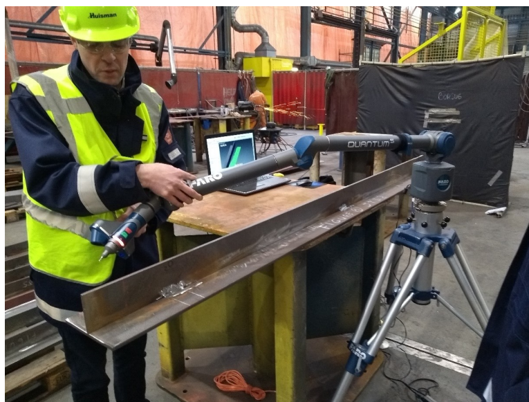
Figure A.3: Scanning of edge geometry with measurement arm
