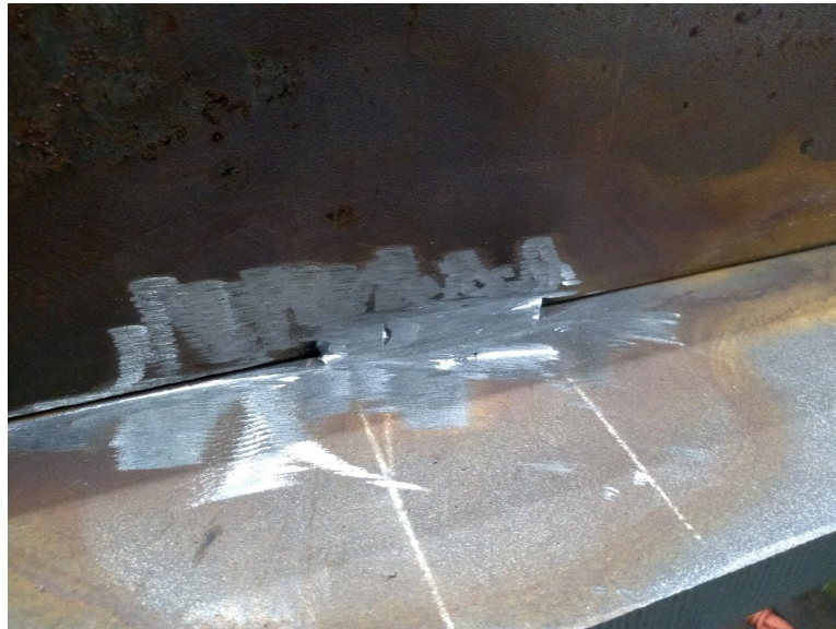
Figure 3.4: One of the three tack welds laid on specimen
