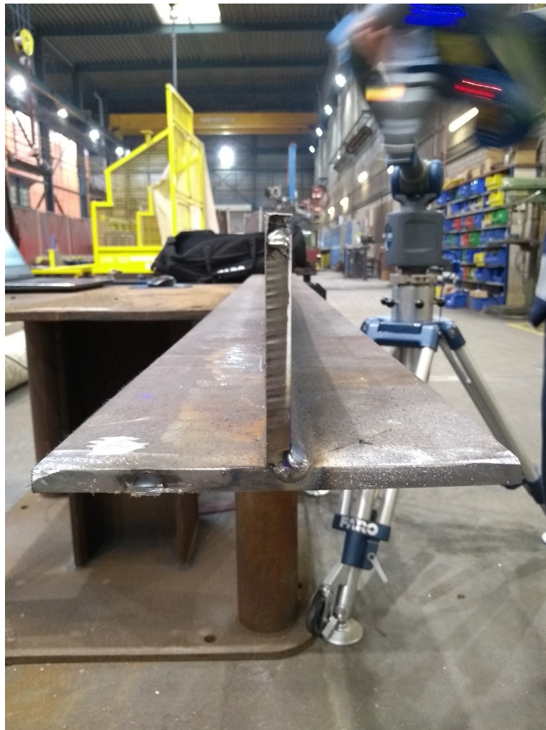
Figure A.8: End of full length weld on specimen
