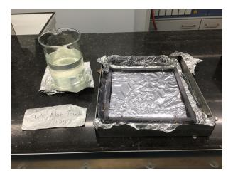
**Figure 3.4:** Coating casting process showing the solidified coating in a beaker and the melted coating in a polycarbonate plate mould inside the metal tray
