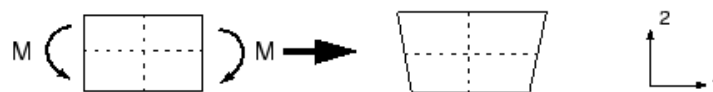
Figure 2.5: Deformation of a linear element with reduced integration subjected to bending moment M [36]
