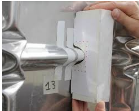
(b) Deformed corrugation
