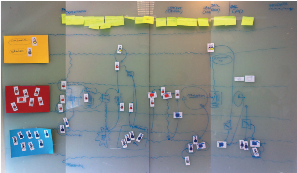
Figure 5.26: The filled in timeline of the design of an ergonomic aerosol, the yellow sticky notes form the preliminary time-line further detailed in the actions mapped on the swim lanes.
