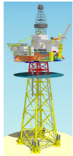
Figure 6: Support Structure with Topside
