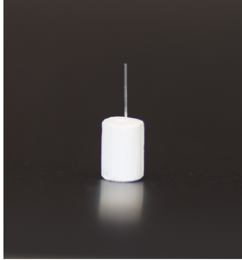
Figure 3: An experimental specimen with embedded PVA fiber
