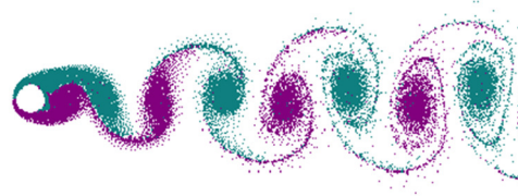
FIGURE 8.2: TURBULENT FLOW BEHIND AN OBJECT IN A STEADY CURRENT, CAUSING VIV
