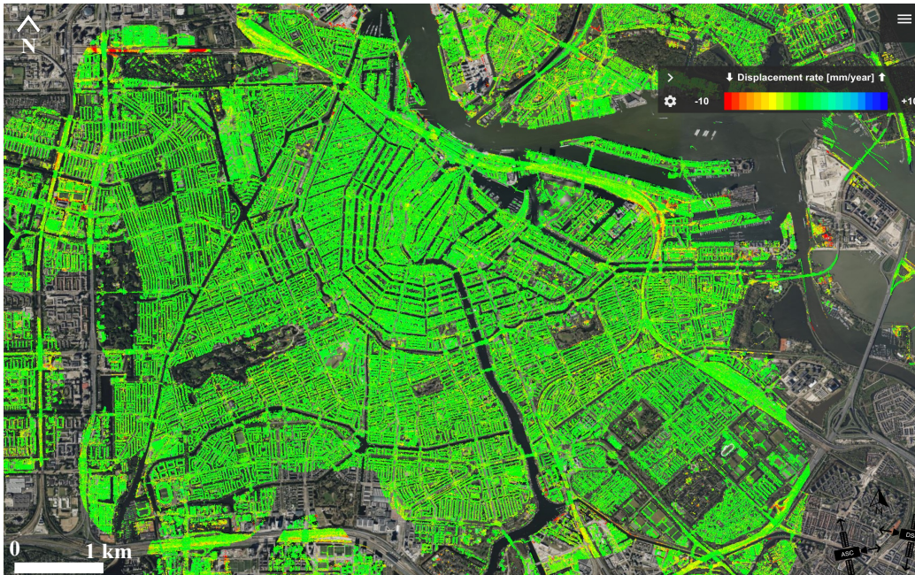
Fig. 1. Velocity map derived from vertically projected MT-InSAR data, as viewed in the SkyGeo dashboard. The map originates from TerraSAR-X descending imagery captured over Amsterdam from 2016 to 2020.
