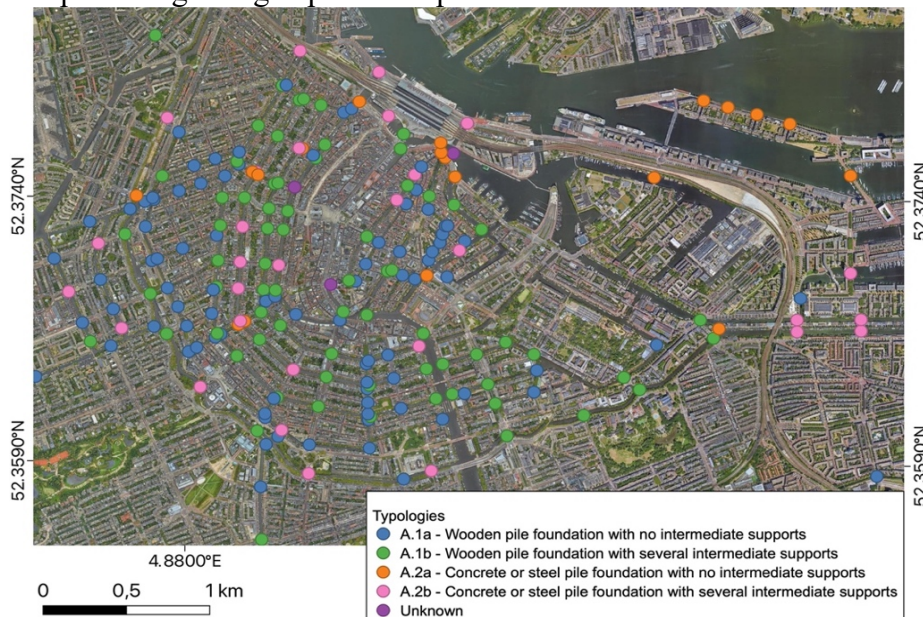
Fig. 2. Bridge typologies in Amsterdam as classified in this study.
