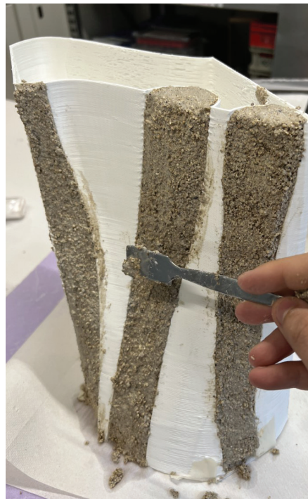
figure 98: : Casting the material inside the cavities (1:3 prototype) (own source)
