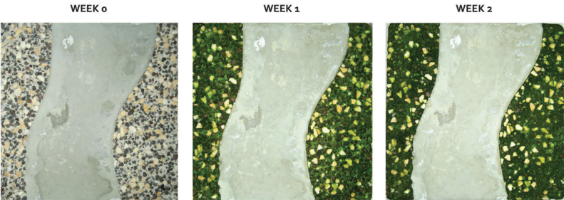
figure 14: Biofilm growth on the bioreceptive part of a concrete panel in a period of 2 weeks. (M.Veeger et al, 2020)
