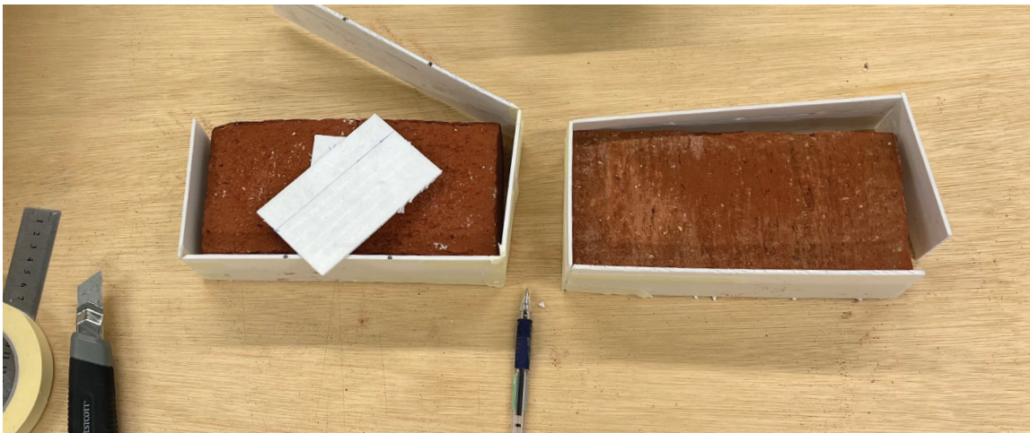
Mold making for mortars using polysterene boards.
