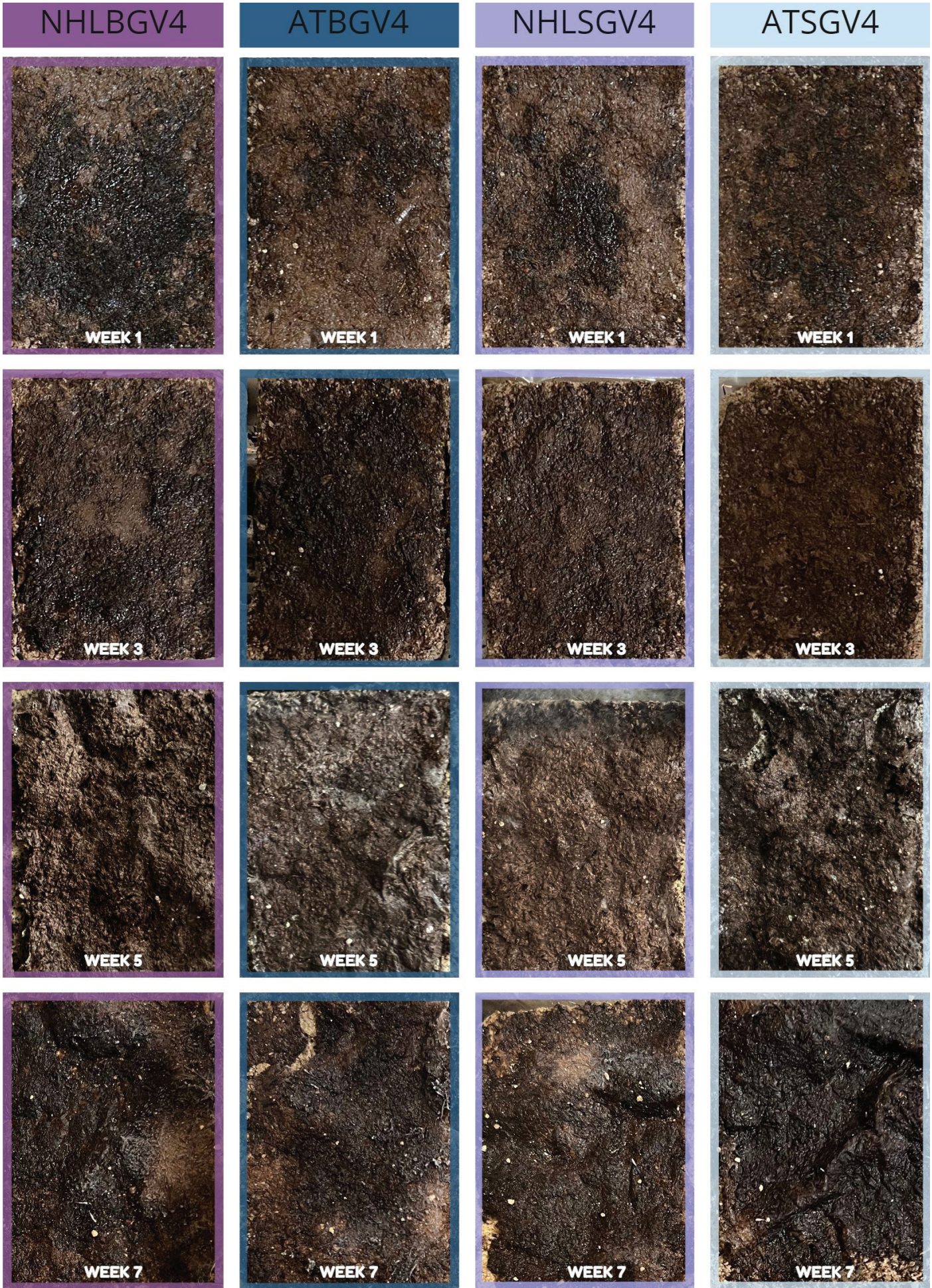
figure 82: Visual observation of the mortars every 2 weeks. (own source)
