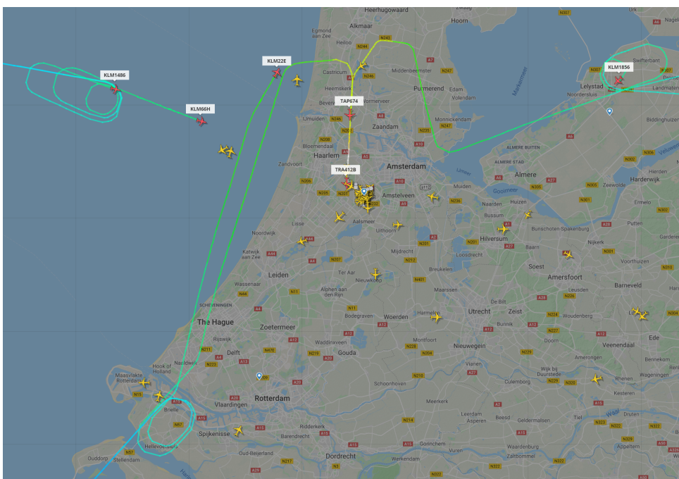
Figure 3.5: Holding stacks for storage above Schiphol airport
