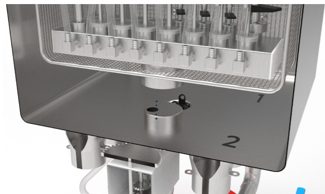
Figure 57: Connecting the lumen basket to the mechanism alternating the flow.
