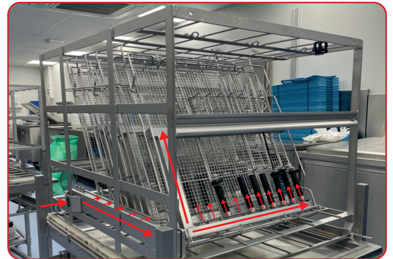
Figure 24: Washer-disinfector rack for cleaning lumens with arrows showing how water flows through.
