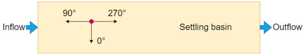
Figure 4.1: Visualization for wind directions used with respect the mud disposal basin in the Delft3D model.
