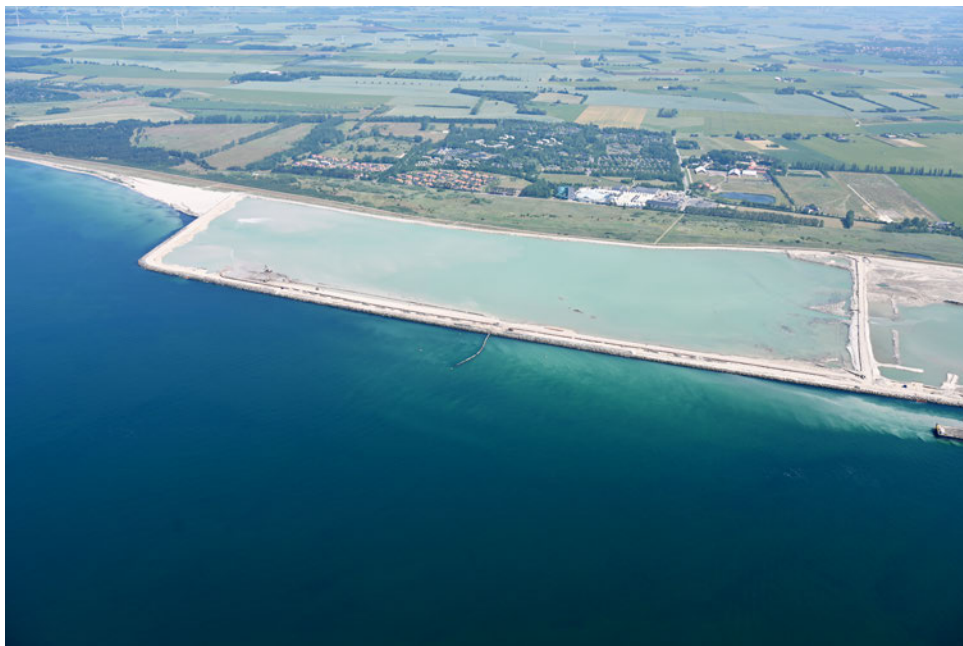
Figure 1.2: A mud disposal basin at the project location of the Fehmarnbelt, Denmark
