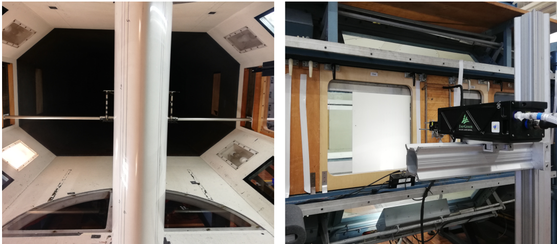
Figure 1. Left: airfoil model on wind tunnel test section. Right: stereoscopic PIV setup for trailing-edge measurements on the airfoil suction side.
