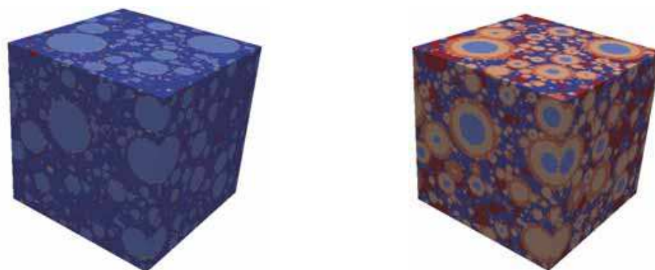
Figure 1: Microstructures of cement paste at –ages of 3 hours (left) and 28 days (right)
