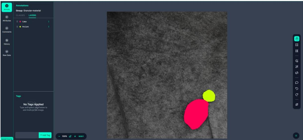
Figure 20 Steps of annotating in images in Roboflow [114]. In order: Loading in an image, create a polygon around the object, assign a class to the object, repeat for all objects and the reference masks for this annotated image.
