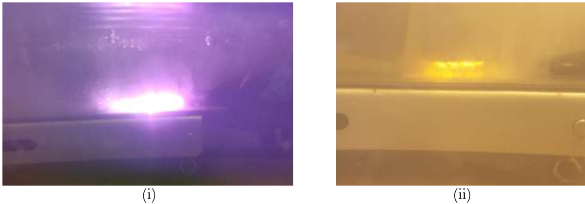
Figure 15 Plasma when the gap is: (i) 1mm, and, (ii) 5mm.
