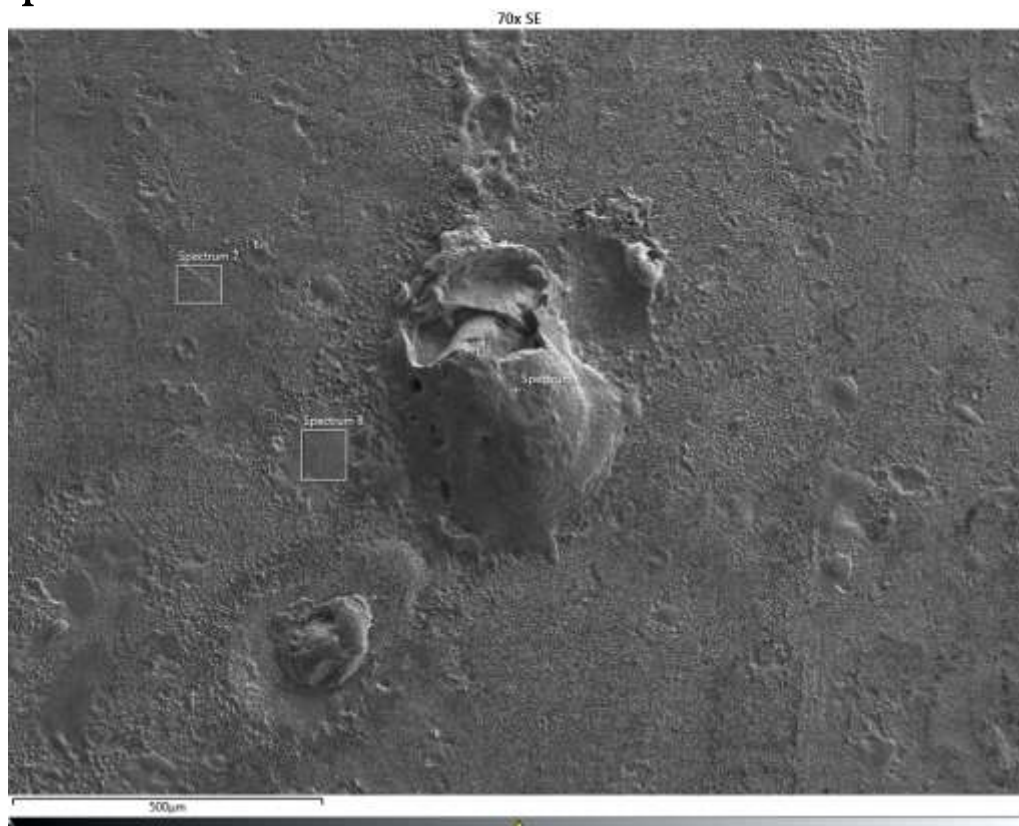
Figure 57 SEM image of Titanium Deposit on DP800 steel surface.
