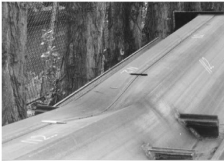
Figure 96: 4-point bending test up till failure of sheet pile [23]
