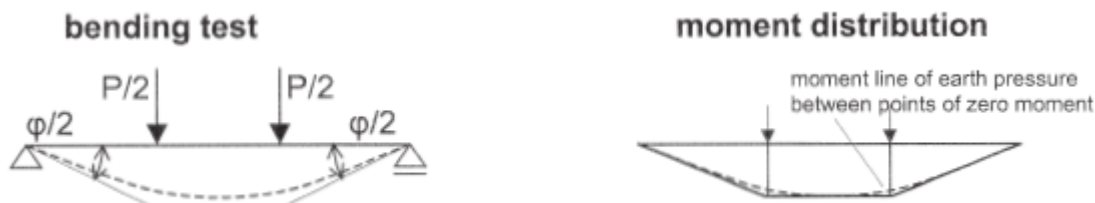
Figure 95: 4-point bending test designed by Sedlacek et al (2001) [30]
