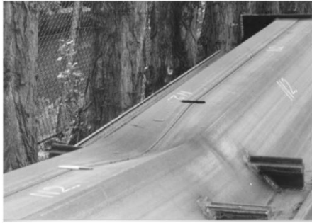
Figure 107: 4-pointbending test up till failure of sheet pile [23]
