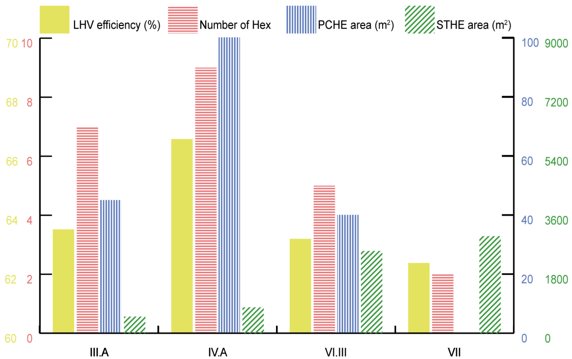
Figure 4.44: Comparison of selected cases (case III.A, IV.A and VI.III) with a directly coupled GT (case VII)
