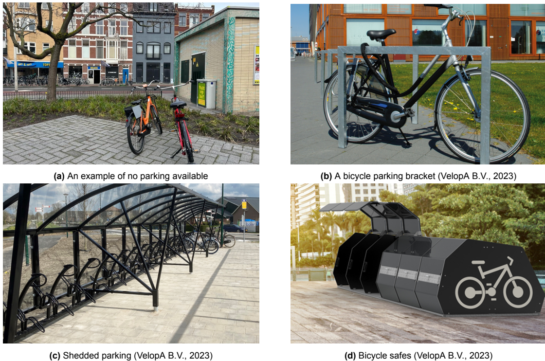
Figure 5.2: The levels of bicycle parking facilities
