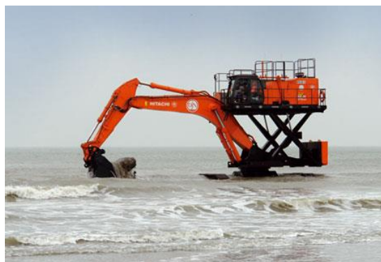
Figure 3-5: Excavator with elevated platform. (Source: bouwmachines.nl )
