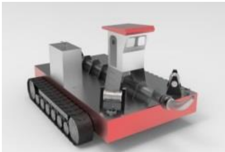
Figure 3-8: A spray pontoon equipped with tracks. (Source: Koen, 2015)
