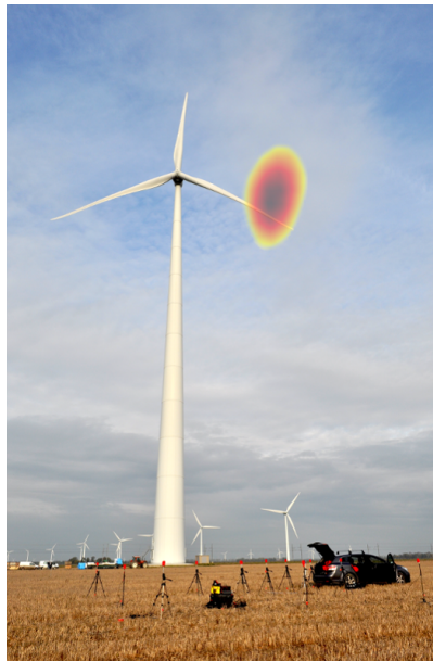
Figure 1.8: Applications of AVS arrays - Sound imaging to localize far-field and low frequency wind turbine noise.
