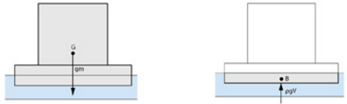
Figure 55- Gravity force and buoyancy force. Source: (Ham,2016)
